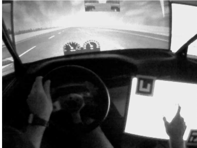
Figure 2. The medium-fidelity driving simulator and the experimental setup from the participant's point of view.
