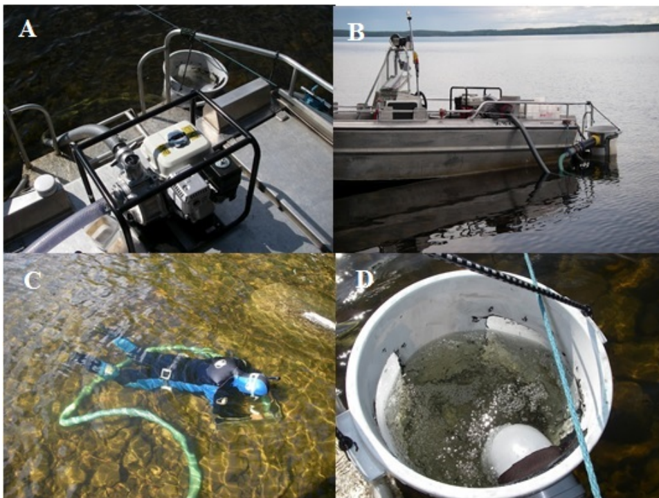
Figure 2. Sampling equipment and machinery: Centrifugal pump (A), the boat (B), snorkeling diver with 0.5 m x 0.5 m frame and pumping up all particles and animals in that surface area (C) and collection bucket equipped with 500 µm sieve (D). Photographs from Kimmo Sivonen.
