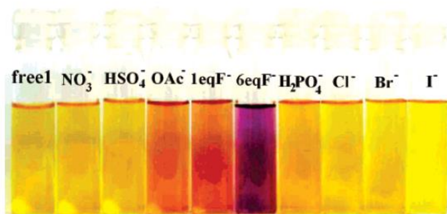
Figure 68. Color change of [\text{Ru}(\text{bpy})_2(\text{H}_2\text{biim})](\text{PF}_6)_2 observed in MeCN solution after the addition of 1 eq. of the corresponding anions as tetrabutylammonium salts (6 eq. for tetrabutylammonium fluoride). 37
