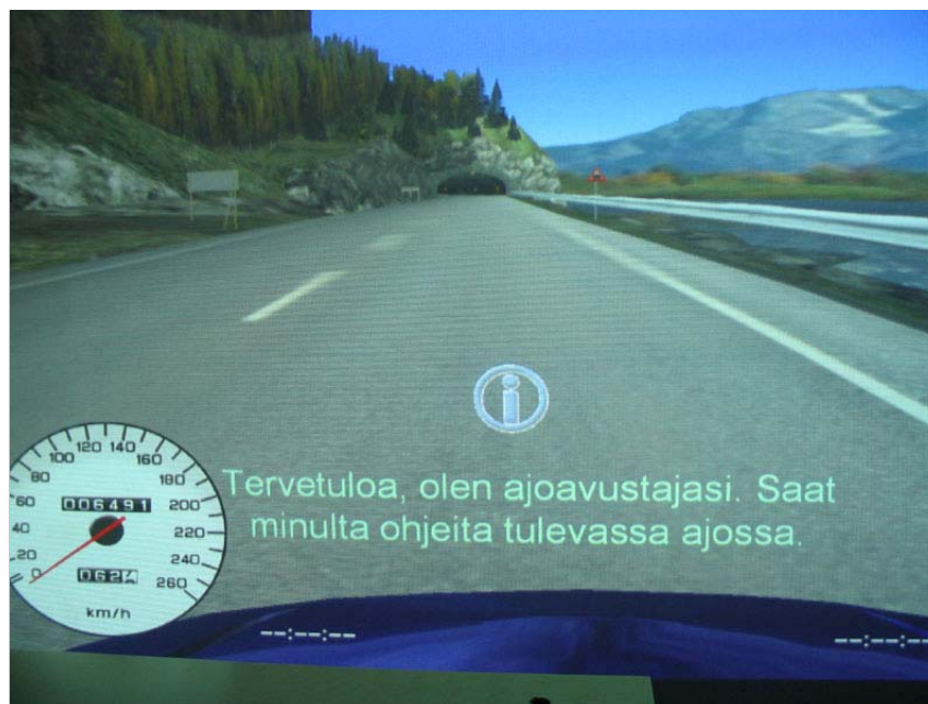
Figure 1. The driver tutoring system with an exemplary tutoring message in Finnish presented in the head-up display.
