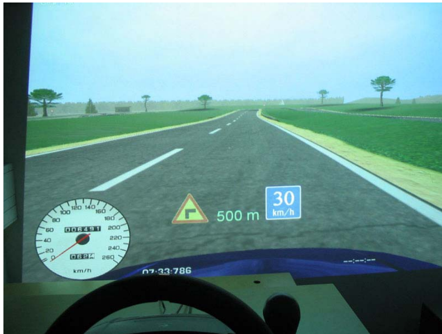
Figure 2. The co-driver system with an exemplary visual message presented in the HUD: in this case, the message indicates that there is a sharp curve to the right in 500 meters and the recommendation speed for the curve is 30 km/h.
