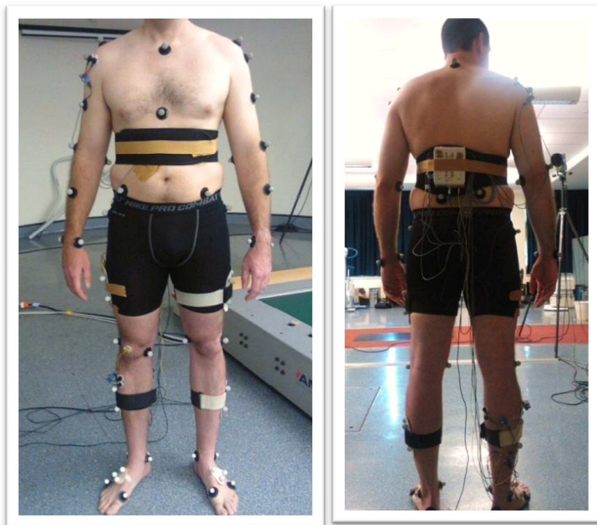
FIGURE 5. Full marker setup with EMG electrodes from anterior and posterior side of the body.
