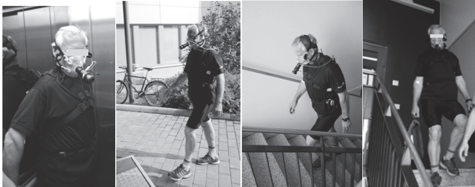
FIGURE 7 Subject performing active and passive transport tests with measurement equipment (portable gas analyser system, heart rate monitor, tri-axial accelerometer and EMG shorts). Pictures from left to right: in the elevator, walking (active transport), stair ascent and stair descent with 5 kg bags in each hand.
