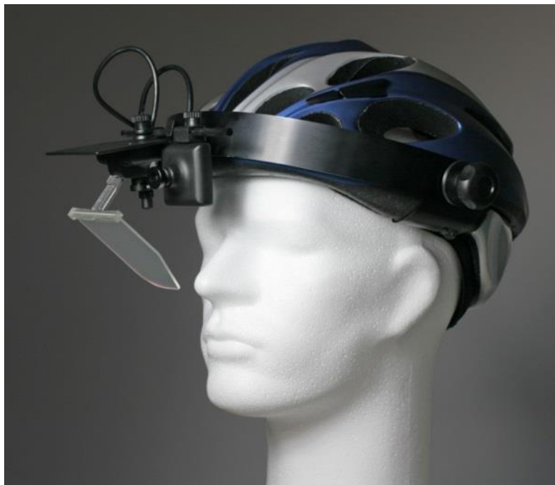
FIGURE 12 SMI iViewX HED 4 device installed in a helmet.
