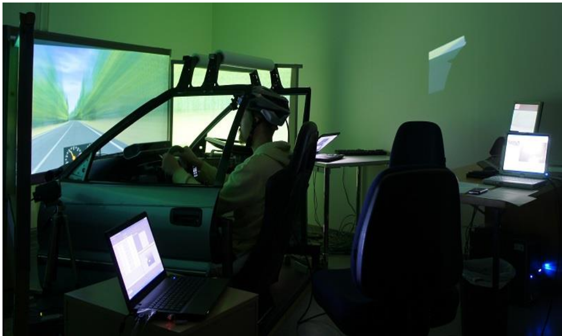
FIGURE 10 Participant driving the University of Jyväskylä Department of Computer Science and Information Systems fixed base driving simulator.
