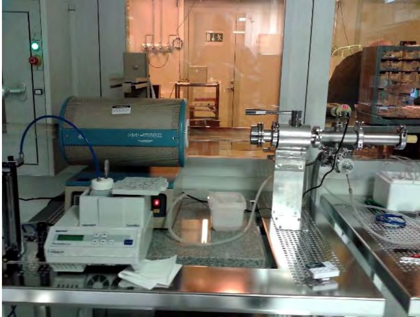
Figure 3.12: CVD system at NSC lab. Tube furnace with 1 m long and 4 cm wide tube element and the load lock system attached on it (On the right). Gas flow meters are seen on the left corner and alcohol bubbler placed in the heat sink of Peltier plate is visible next to those.
