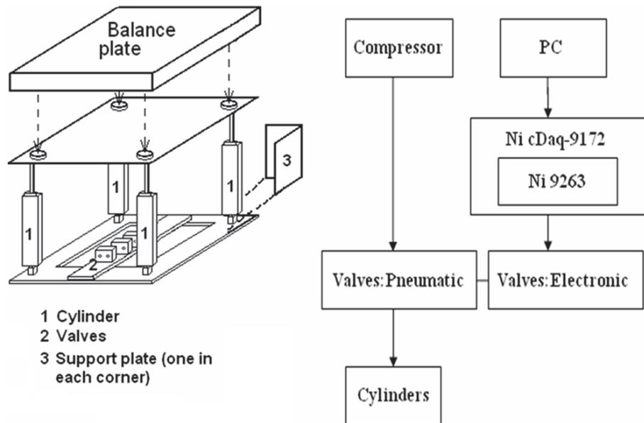
FIGURE 4 Vertical dynamic balance measurement system and flow chart.
