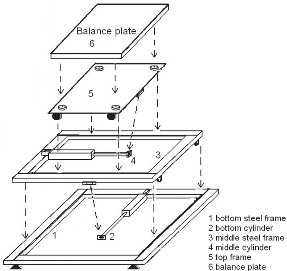
FIGURE 5 Horizontal dynamic balance measurement system. The bottom cylinder moves the middle frame in the anterior-posterior direction, and the middle cylinder moves the top frame in the medial-lateral direction.
