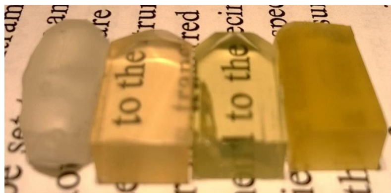
Figure 5.10 Visual transparencies of some epoxy composite blocks with different silica contents/surface modifications. From left: 1 wt-% bare silica, 2 wt-% silica-PGMA, 2 wt-% silica-PGMA-oligothiophene and 4 wt-% silica-PGMA-ferrocene in epoxy.
