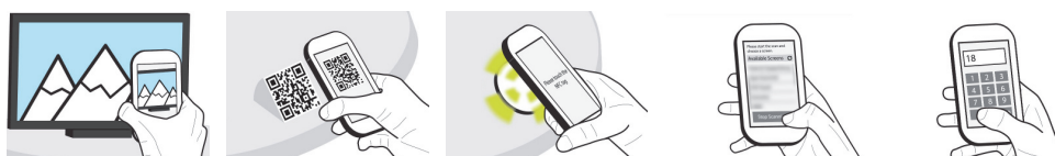
FIGURE 4 PMI techniques. From left: pointing (image recognition), pointing (QR codes), touching (NFC), scanning (Bluetooth), manual input (text typing)
