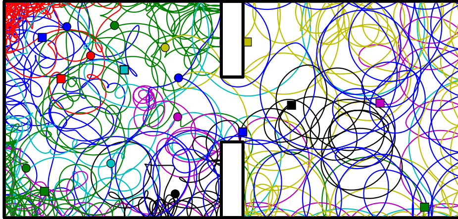
Figure 30: With effective Larmor radius r_{\text{ELR}} = 0.103 the magnetic field strongly bends the particle trajectories and therefore increases the average relaxation time compared to larger r_{\text{ELR}} .
