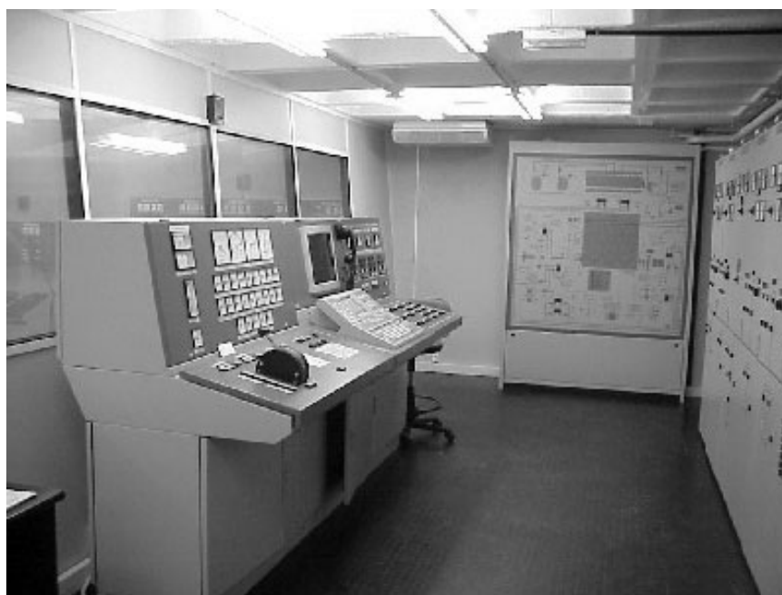
FIGURE 2 Overview of the HF MCRS equipment and environment used in Experiment 3 by the HF group throughout the experiment. The LF group used this equipment only in the transfer phase. From the remote control console, on the left, only the CRT display and the keyboard in front of it were used. The local control panels are located in the contiguous room to the left of the console (visible through the window).
