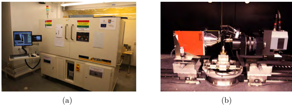
Figure 19. a) Xradia MicroXCT-400 and its b) X-ray source (20 – 90 kV) (on the left), sample holder (in the middle) and optical lenses (on the right).
