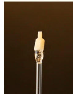
Figure 18. A fully prepared sample ready for scanning. It was defrosted, ground and glued to a glass capillary. Imaging was done of the small tip of the sample.
