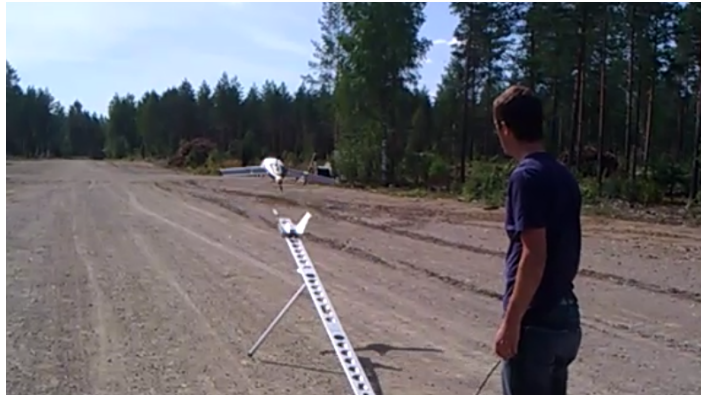
Figure 5. Gatewing X100 UAV launched with catapult to acquire airborne images.
