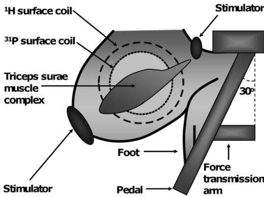
**Figure 1. Schematic representation of the setup for measuring rat triceps surae muscle complex function with MR investigation.** Triceps surae contractions were induced indirectly via electrical stimulation at the heel and knee levels. Muscle performance was measured with a force transducer which was attached to the pedal. Information about the leg position was acquired with a <sup>1</sup>H-MR surface coil and muscle metabolic functions were studied with <sup>31</sup>P-MRS surface coil.
