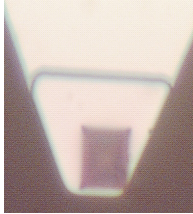
FIGURE 2.5 Misaligned tip causes mechanical cross coupling. The tip is about one micrometer off the centerline of the cantilever. The image is taken with an optical microscope.
