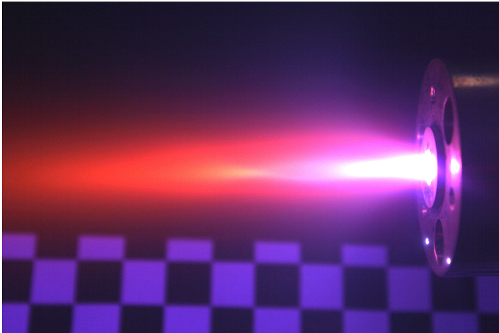
Figure 5.6. A photograph of the slightly underexpanded gas jet of argon emitted from the new de Laval nozzle. Using the 1 cm by 1 cm checker board in the background, the jet length can be estimated to be \sim 9 cm with a width of \sim 6 mm if one disregards the halo around the shock structure.
