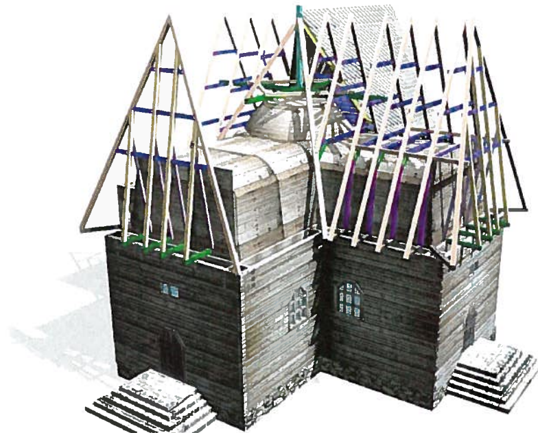
Figure 6. The roof structure of the Church of Petäjavesi. Different colours are used to illustrate structures.
