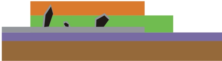
Figure 3.3. Sample schematics. Pinholes and particles in the insulating SU-8 layer are shown in black. In this configuration there is a short from top electrode to the bottom.
