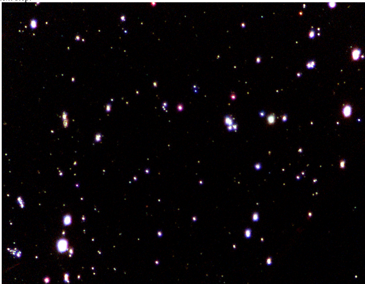
Figure 3.2. The surface of the Si chip after wet cleaning. Dark field optical micrograph, 20X.
