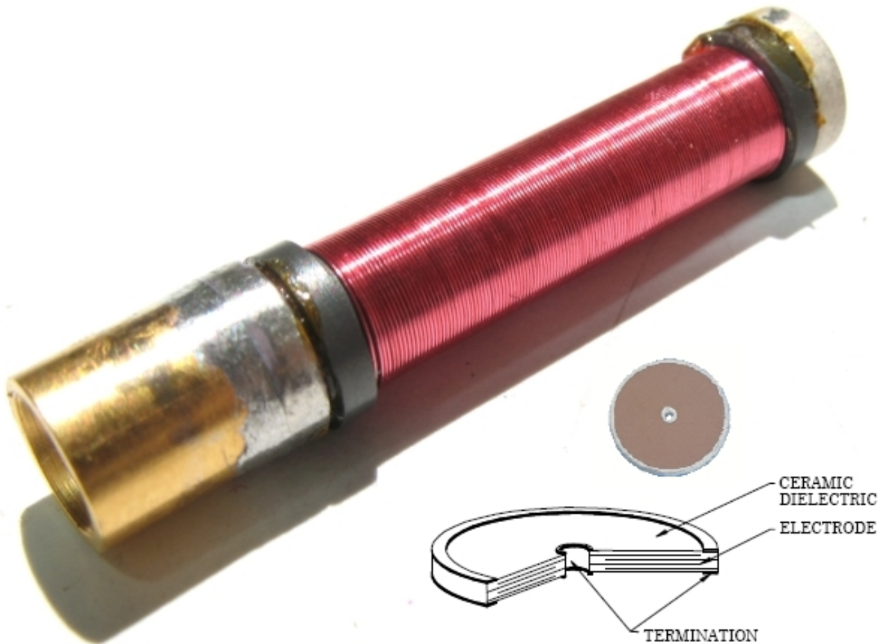
Figure 2.4. Filter core with copper coil, two capacitors and one MCX connector. The schematic picture of the discoidal capacitor is also shown (capacitor image is taken from the PA&E official catalog).
