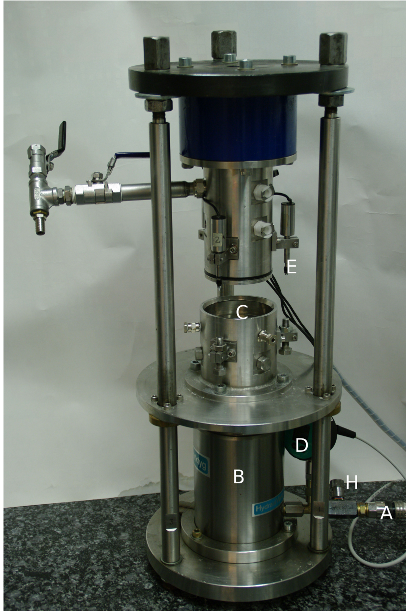
Figure 3.3: The compression device for the one-dimensional constrained compression experiments. The letters refer to the same components as depicted in figure 3.2.
