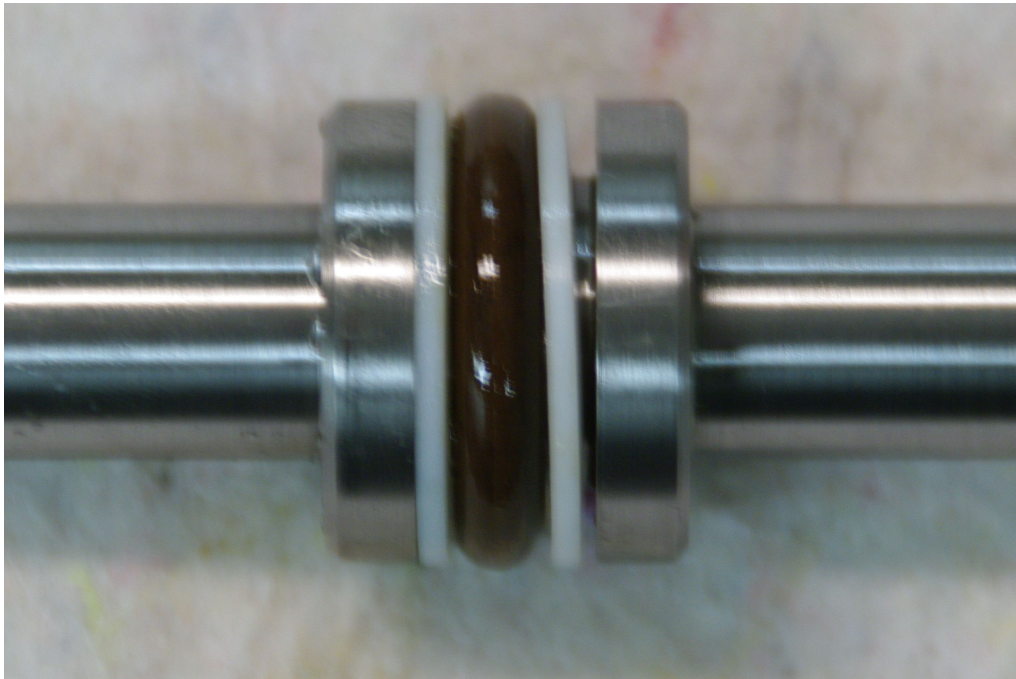
Figure 4.7: A photo showing the axis of the double action hydraulic cylinder after the measurements had been completed. A relatively large gap can be seen between the seals and the edge their mounting groove. This gap allowed the seals to move back and forth during the measurements, possibly causing the poor repeatability.
