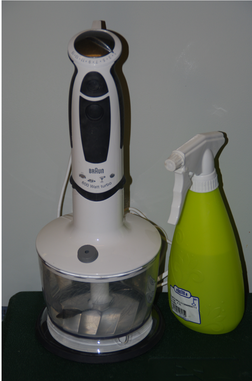
Figure 3.1: The primary equipment used in adding and mixing water with the clay.
