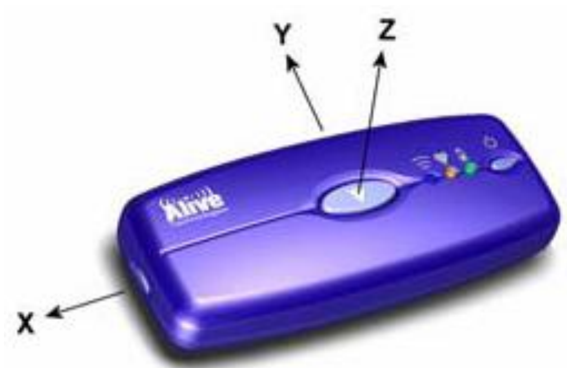
FIGURE 9. Alive Accelerometer and orientation of x, y and z axis (Alive manual 2006).
