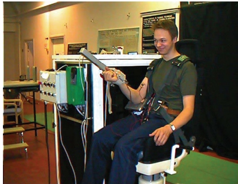
FIGURE 2 The eccentric exercise test arrangement in an isokinetic machine (Komi et al. 2000)
