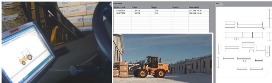
FIGURE 21 User interface of the smart wheel loader working in the outdoor warehouse area of wooden products
