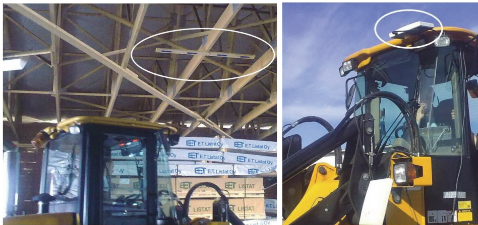
FIGURE 26 RFID-based navigation of a transporter inside the warehouse
