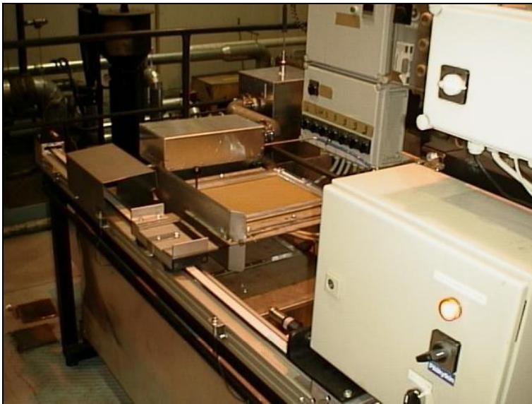
Figure 23. Combo system in the impingement drying mode.
