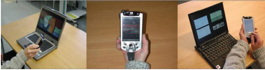
FIGURE 22 The video is streamed to the laptop (left), followed by a session handover to the PDA (center), and a handover back to the laptop (right)
