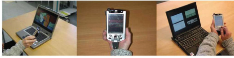
Fig. 4. Triggering in practice. The video is streamed to the laptop for the first three minutes (left), followed by a session handover to the PDA (center), and a handover back to the laptop (right).
