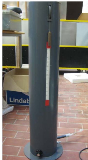
Figure 9.11 Calibration device of flowmeter
