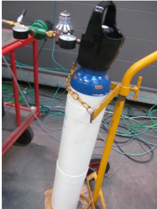
Figure 9.8 Bottle of N 2 O connected with manometer
