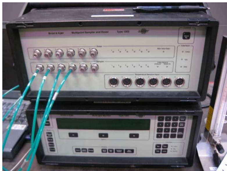
Figure 9.9 The tracer gas measuring devices
