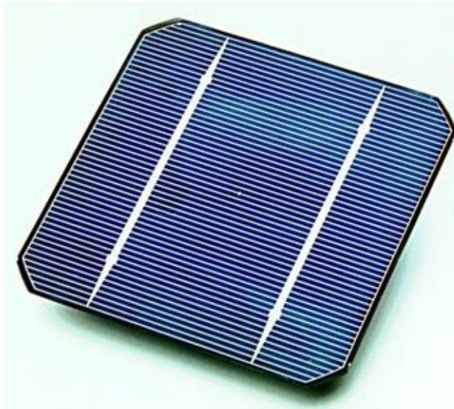
FIGURE 4: Solar cell made from a mono-silicon wafer [9].
