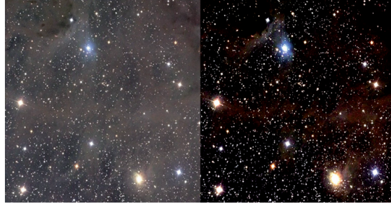
FIGURE 34 Fractional diffusion based deconvolution (right) for \sigma_n/\sigma_{I_0} = 1 of a dust clouded star field (left) in the constellation of Pegasus.
