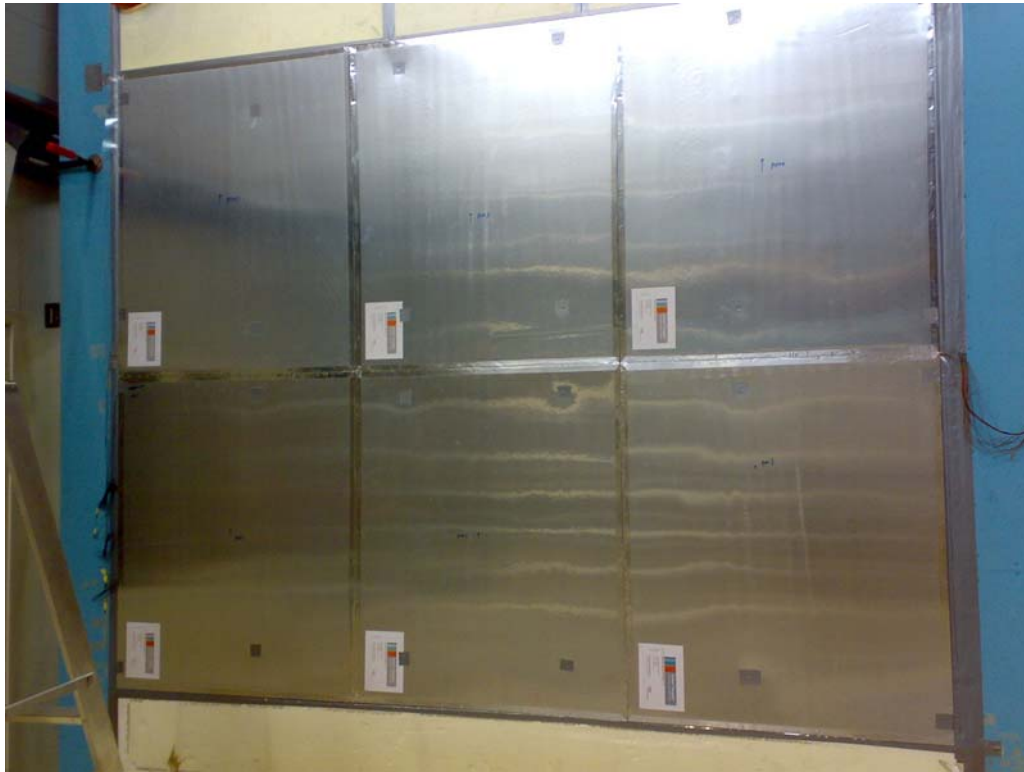
Figure 4.21. A photo taken after attaching the Dupont™ Energain® PCM panels onto the surface of vapor barrier.
