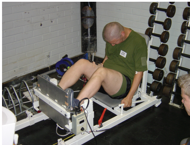
FIGURE 3 Measurement of maximal isometric force of the bilateral leg extension with an electromechanical dynamometer.
