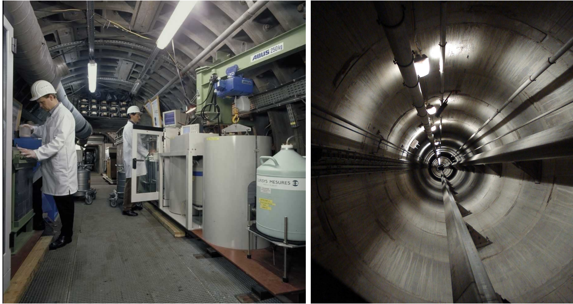
Figure 3.2: On the left is IRMM's ultra low-level \gamma -ray spectrometry laboratory in HADES and on the right a view down the elevator shaft, 223 metres deep. The Research Group Leader, Mikael Hult, is working on the left in the photo of the HADES \gamma -ray spectrometry laboratory.
