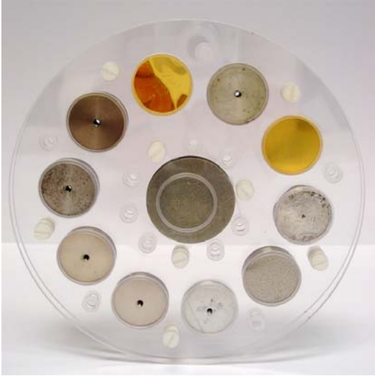
Figure 1. Photo of the second-generation neutron detector unit. The overall diameter of the detector unit is 120 mm.
