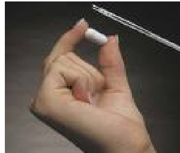
FIGURE 4. The comparison of the size between a telemetry pill and a classical thermometer.
