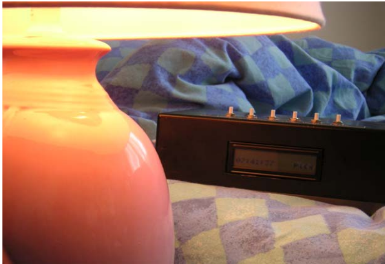
Figure 7. The control interface unit developed for the X10-based home automation prototype system. The unit was a black box, approximately the shape and size of a common clock radio, with several buttons and a LCD screen available for users to make changes to the morning and evening time presets of the home automation system.
