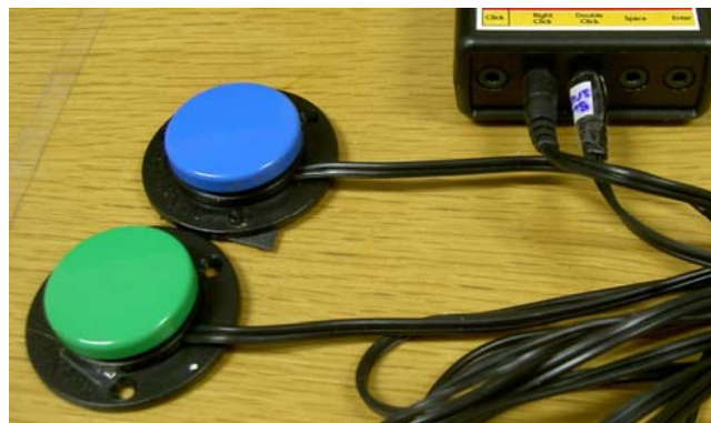
Figure 3. Switches with a PC interface box.
