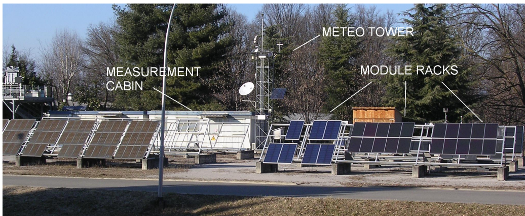
Figure 16: The outdoor measurement field of ESTI at the JRC in Ispra, Italy.
