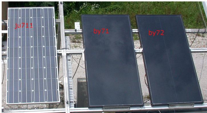
Figure 31: The studied modules: one c-Si module and two CIS modules, denoted by ju711, by71 and by72, respectively.
