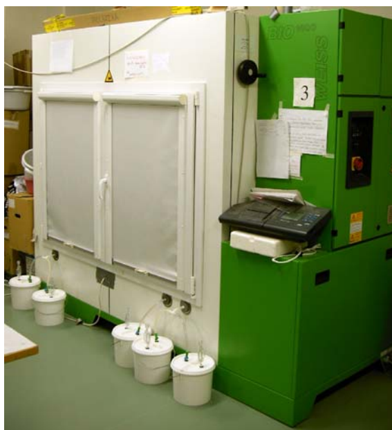
Figure 1. Growth chamber Bio 1600 Weiss in operation with visible outlet absorption apparatus. The tests were not influenced by room lightning or room temperature.
