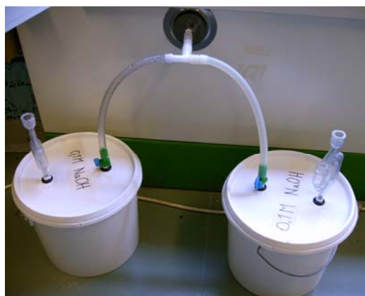
Figure 4. The outlet, VFA containing, air from the growth chamber was purified by absorption to 0.1 M NaOH solution, when bubbled through liquid containing tightly closed, water lock bearing 5 liter buckets.
