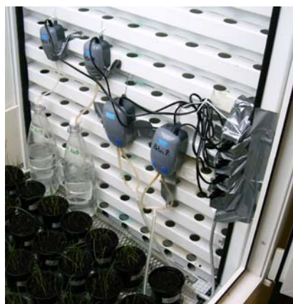
Figure 3. Closer look at the inner pumping and absorption apparatus in growth chamber.
