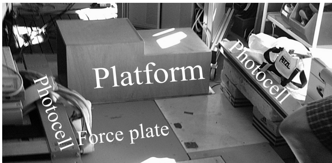
FIGURE 5. The setup for drop jumps.
