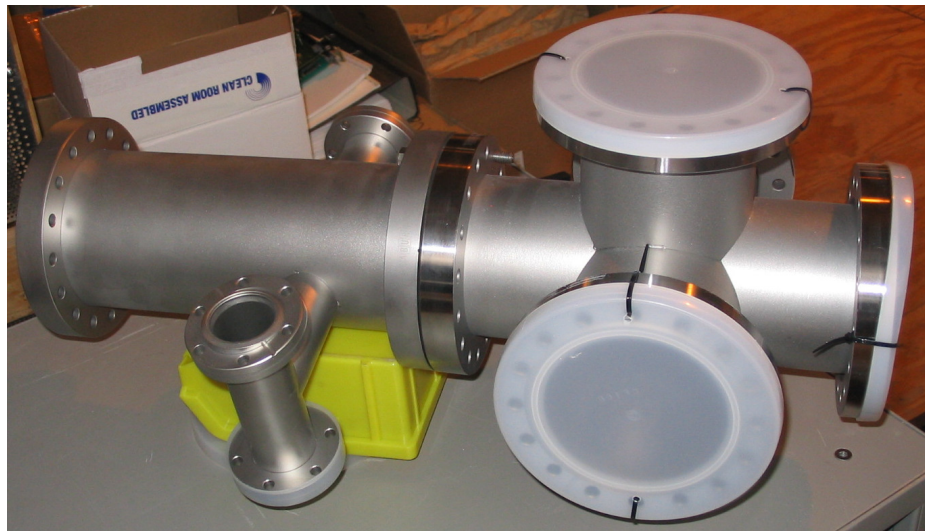
Figure 6.11: The lower cross with the extension piece to enable the connection of a pump and pressure gauges.
