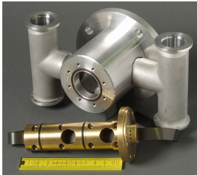
Figure 6.8: Differential pumping/slit system to guide the tape into vacuum developed by Wilfried Hüller at GSI.
