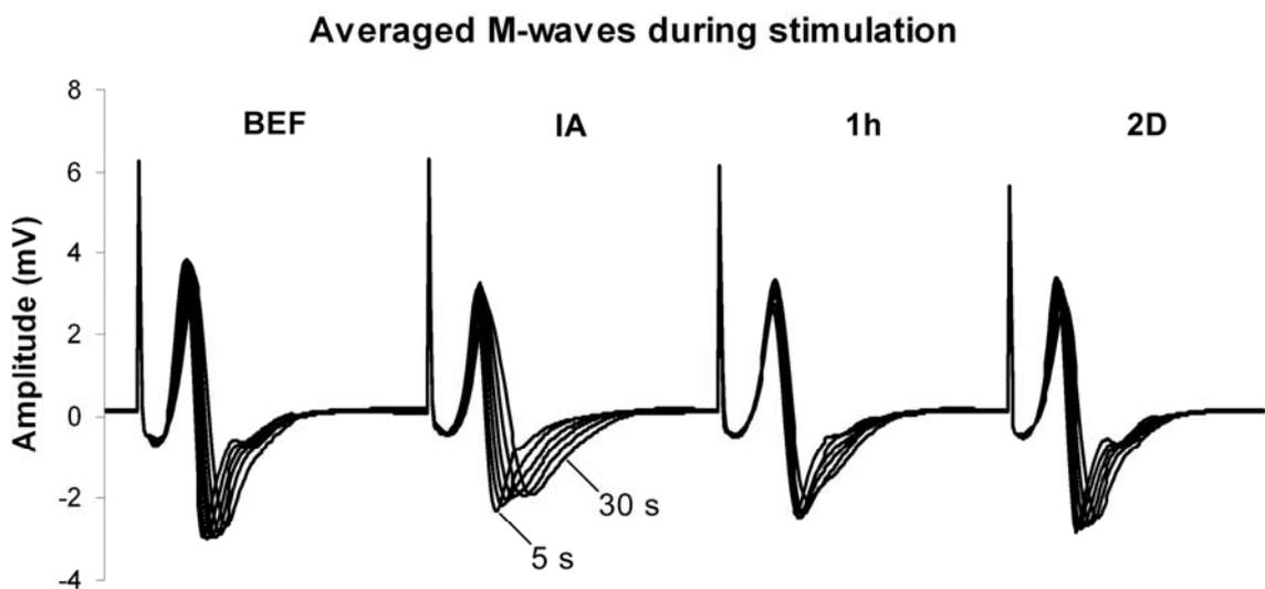
**Figure 11.** An example of six superimposed M-waves with 5 s intervals during tetanic stimulation from one subject.
