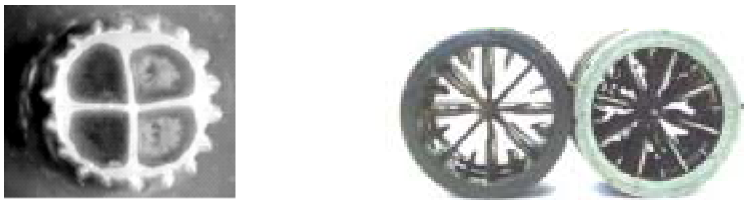
FIGURE 1 Biofilm carriers used in suspended carrier biofilm processes. Left: Kaldnes KMT carrier used in laboratory, diameter 10 mm. Right: Flootek RF 438 carriers used in pilot studies, diameter = 44 mm.
