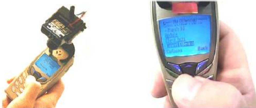
FIGURE 9. Mini-camera, which was attached to the phone (left) and the view that it videotapes (Nyyssönen, Kaikkonen & Roto, 2002). It should be noted, that the phone and the view are not related to our experiment.
