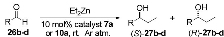
Scheme 10. Model reaction of diethylzinc with aromatic aldehydes. Reactions and conditions: Et 2 Zn, 10 mol% catalyst, n -hexane, Ar atm., rt, 20 h, b : 4-MeC 6 H 4 , c : (4-MeO)C 6 H 4 , d : (3-MeO)C 6 H 4 , 80–90%.
