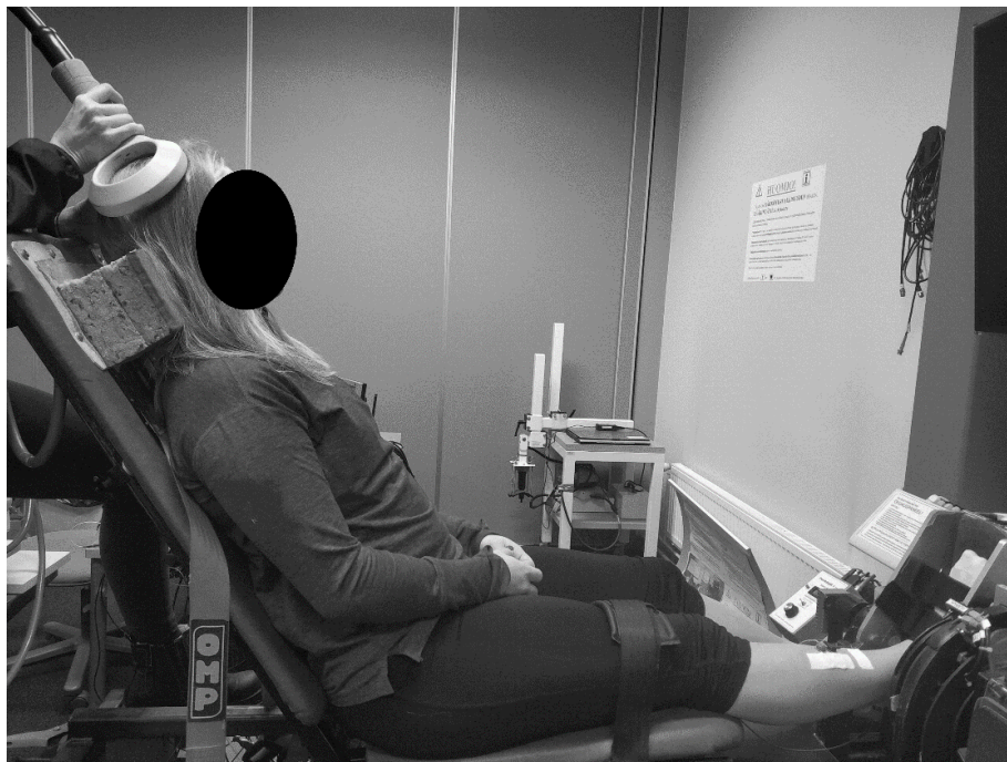
FIGURE 8 Measurement setup and subject position in Experiments III. The subject sat on a custom-built ankle dynamometer during the experiment.
