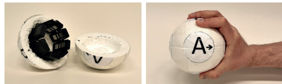
Figure 2: Left – Carved open polystyrene ball with the Myo armband in it. Right – Closed ball.
