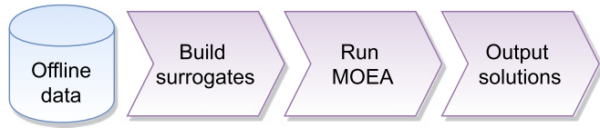
Figure 1: Flowchart of a generic offline data-driven multiobjective optimization approach.
