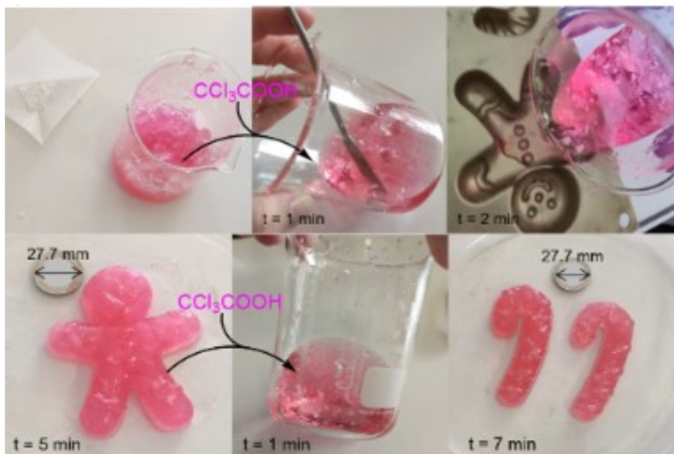
Figure 27. Reconfigurable objects made from transient TCA-fueled gelation system. The gel-sol-gel system could be reproduced about 15 times. 8 Reprinted with permission from ref. 8. Copyright 2022 American Chemical Society.
