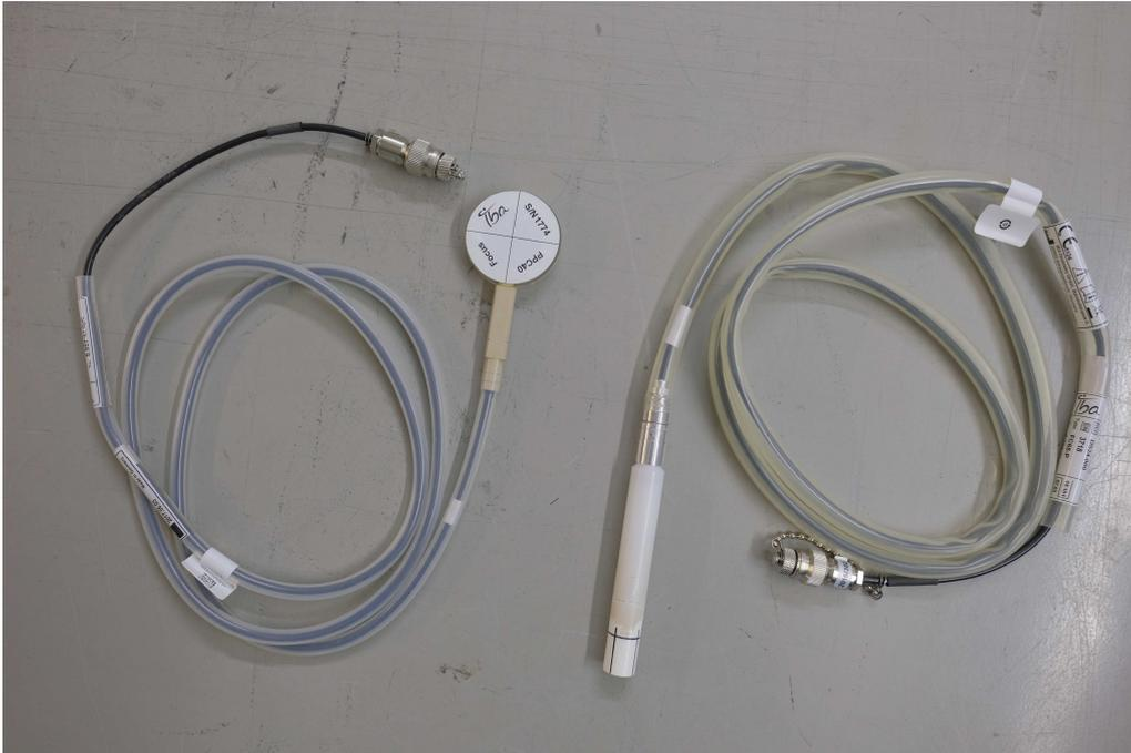
FIGURE 8 Photograph showing a parallel plate ionization chamber to the left, and a Farmer type ionization chamber to the right. The Farmer chamber is covered by a protection cap (build-up cap), inside of which the cavity is located. For reference, the diameter of the top view of the white parallel plate chamber surface is 42 mm.
