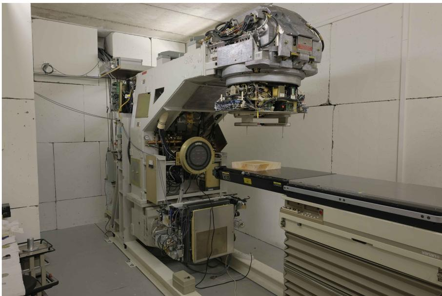
FIGURE 12 A photograph of the RADEF Clinac. The beam direction is downwards in the picture, coming from the accelerator head towards the so called couch where a block of acrylic can be seen in the beam window position.
