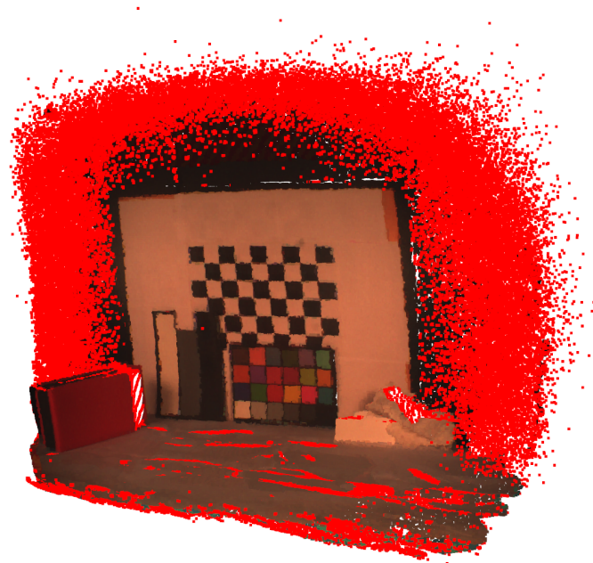
Figure 6. Visualization of the outlier removal for the point cloud in the middle camera viewpoint. The points highlighted with red were removed.
