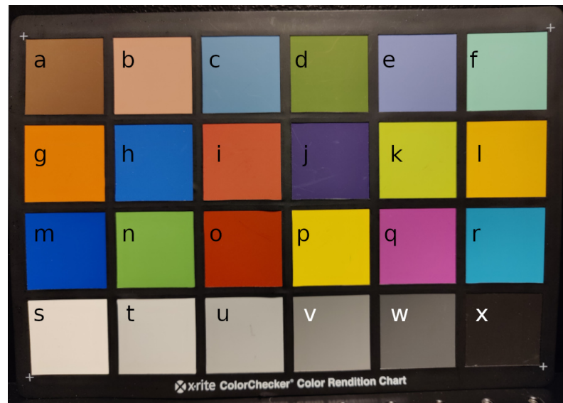
Figure 12. The color checker board used for calculating the result reflectances. Letters a–x correspond to each tile and a result plot in Figure 11.
