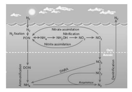
Figure 1. Marine N cycle. PON = particulate organic nitrogen, including phytoplankton; DON = dissolved organic nitrogen, DNRA = dissimilatory nitrate reduction to ammonium (Arrigo 2005).
