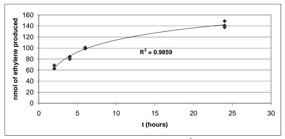
Figure 7. The production of ethylene in darkened bottles. The  $R^2 = 0.9859$  when the trend line is logarithmic.
