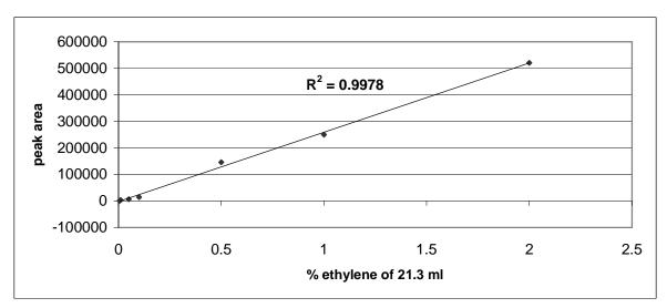
Figure 4. The correlation between the peak area and ethylene concentration
